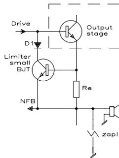
In Figure 5.19, the emitter degeneration resistor  $R_e$  in the output stage develops a voltage across it in proportion to the output current in this half. The output current is clamped (or limited) at the current where this exceeds the current required to turn on the limiter BJT (a small signal part) hard enough to divert any further drive.
