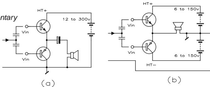
Figure 4.10 shows the all-common-emitter (CE) type, with a single supply (a) and with dual supplies (b, c) with different grounding arrangements. With the superficial similarities, confusion is easy. To distinguish between CE and CC (follower) stages, look to see if the speaker is (or would be) *connected between the emitters of the output transistors and the input signal reference* (ground). If so, the stage is a follower (CC); if not, it is CE.
