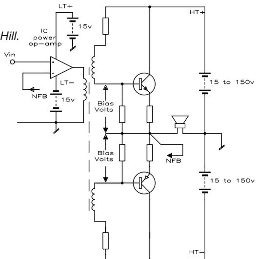
had plagued most direct-coupled amplifiers in professional use in the early 70's, when the circuit was conceived. The transformer also keeps any DC offset voltages (from the driver stage) out of the output stage, and thence from affecting the biasing. The alternative would be four blocking capacitors.
