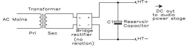
The small disadvantage is that rectification is also performed in (its own) true bridge configuration, where two rectifier diodes are conducting in series at all times. This doubles the small rectifier losses, compared to the dual supply (Figure 6.1) with dual, bi-phase rectification, where the current for each polarity passes through only one rectifier diode at a time.
