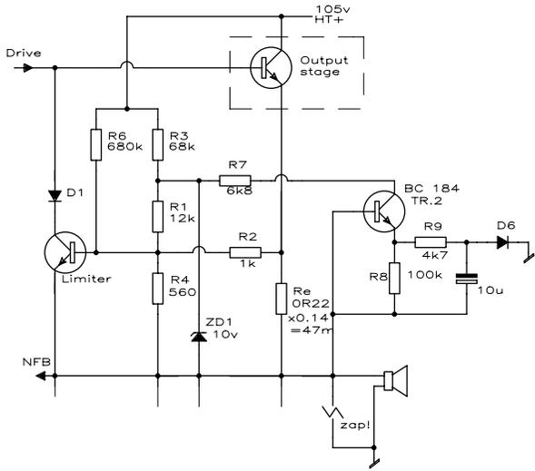
used, comprises seven paralleled power transistors, the effective value of  $R_e$  is about  $47m\Omega$ , if each leg resistor is  $0R33$ .
