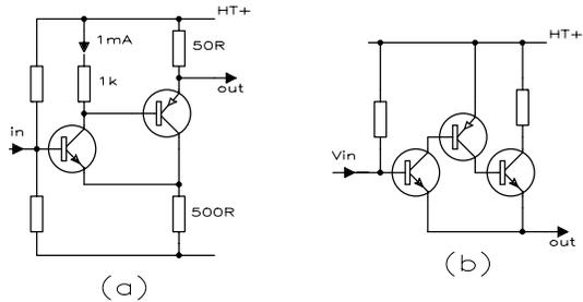
The *triple* (tripp'ull') is a mega-transistor built from three BJTs, and the natural progression of the Darlington. Figure 4.22 (a) shows the most obvious format – as still used by Crown. The sizes of the transistor symbols are a symbolic reminder that even more than with the Darlington, the transistors in a triple are cascaded in their current handling and capability, i.e. small, medium, then large.
