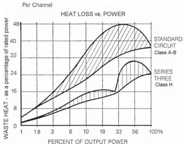
*signal levels averaging*  $>5\text{dBvr}$ , i.e. above 30% of full power. If the signal is compressed, clipped or bassy enough for this kind of condition to be prevalent, then the difference is a significant one: At 56% of full power (2.7dBvr), Carver quotes 65.7% whereas QSC's curve is indicating 76% with sine waves, and 82% with music drive. But with substantially uncompressed music and speech, i.e. purer live sound, the difference recedes.
