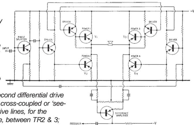
One reason to choose the bridge was the recognition that as with a push-pull stage (in the normal half-bridge), bridging cancels asymmetric differences – which create *even-order* harmonic distortion products. The foremost cause of such differences, at the time, was that between nominal *pnp* and *nnp* ‘complements’. Bridging excised these bugging little asymmetries. It seemed elegant at the time.
