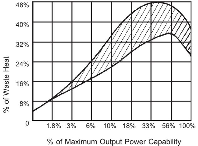
When driven at their rated maximum power, real class B amplifiers are plausibly efficient at 74%, compared to 78.5% predicted by first-order theory, which is ignorant (for example) of bias current. The graph also clearly shows how continuous sine-wave testing at about one third of full power delivery is the acutest bench test of a class A-B amplifier's heat dissipation capability.
