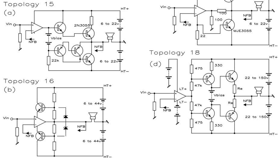
safe limits if the supplies are able to approach or exceed double the op-amps' rated voltage. In this drawing, the op-amp may be *any* power stage with split rails and a differential input. If only a low power op-amp, a current gain (output) stage would be interposed. If a power stage, we have a *supertopology*.
