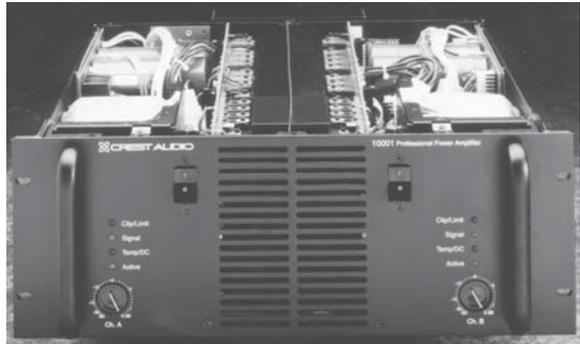
*ratings, that individual hosepipe-sized power cords are fitted per pair of channels - hence the two power switch/breakers seen here. Notice the central tunnel cooling, and the general symmetry of the weight disposition, with end-on toroids up front, and reservoir capacitors behind. © Crest Audio Inc.*
