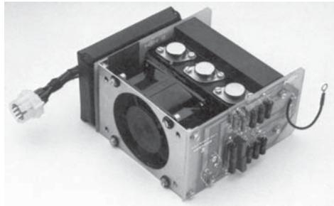
Today, some aspects of heat exchange can be readily modeled on an analogue circuit simulator, with R-C networks, with  $T_{\text{amb}}$  as a current source, etc. Each obstacle in the way between the waste air and the transistor junction is a resistor.
