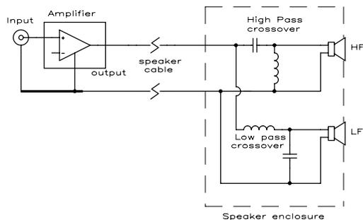
In this form, the crossover comprises physically large and heavy, high voltage-rated capacitors, high current-rated inductors (coils), and high power-rated resistors.
