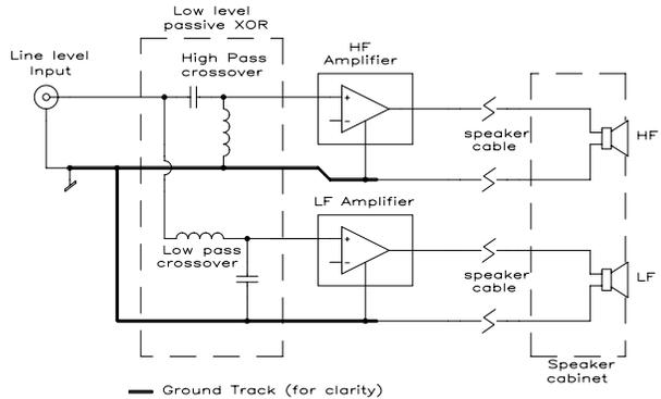
Otherwise, in ordinary ‘mix and match’ sound systems, one problem arising is that the crossover is physically divorced from the speaker, so careful connection is needed. Another, less daunting, is that any existing, passive high level crossover component values cannot be simply transferred, since they will have been ‘tweaked’ to best suit the vagaries of the drive-units’ impedances.
