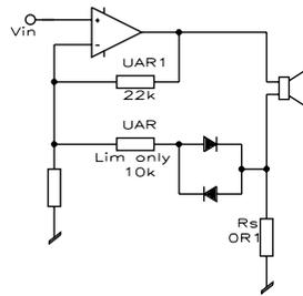
The next generation of transistor protection was more subtle, as circuitry which limited current alone developed into ‘Load line-limiting’ or Load line protection’ alias ‘V-I limiting’ or ‘V-I protection’; they are all the same. The following figures 19 to 26 cover the evolution.
