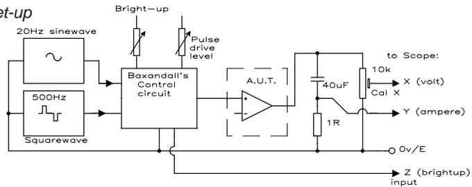
transient effects and protection circuit action, was published by Peter Baxandall [17]. Baxandall's circuit (Figure 5.30) drives the amplifier into hard but very brief clip, with  $50\mu\text{S}$  pulses on the back of a 20Hz sine wave. This enables the limits into reactive loads in particular, to be fully explored without stressing or destroying the amplifier, and with relatively little dissipation in the test load either.
