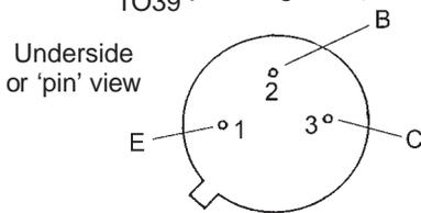
Pin 3 is connected to case
