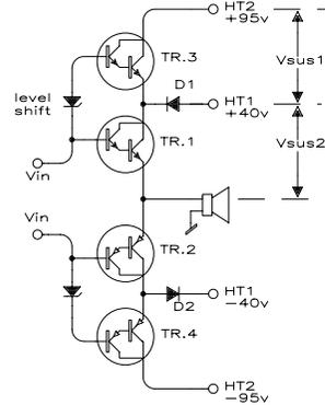
The outcome is cooler running, than if TR.3,4 with their  $\pm 95\text{v}$  rails, were passing current all the time. In effect, switching is being used to improve efficiency within an analogue amplifier.
