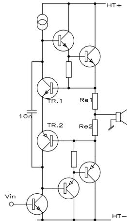
This same scheme also offers protection against short circuits, required with this push-pull output stage topology. Note that no such protection is required for the single-ended schemes that are biased by a constant current source – just so long as the current source controls itself against temperature.
