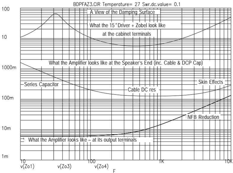
ability is degraded to, after it has traversed a given speaker cable and passed through an ideal  $10,000\mu\text{F}$  series capacitor, as commonly fitted in many professional cabinets for belt'n'braces DC fault protection. The rise at 1kHz is due to cable resistance, while cable inductance and the series capacitance cause the high and low-end rises respectively above 100 milliohms.
