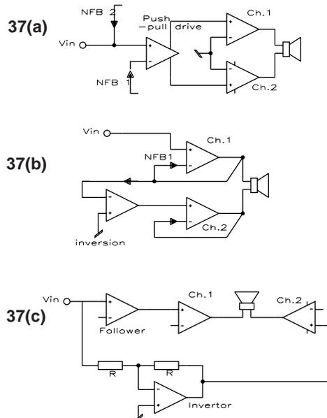
currents will pass through the ground system, and distortion may worsen and will certainly change, as a result. Figure 4.37 (c) shows the more refined method, where the push-pull or differential signals for both sides are derived in parallel, and at line signal levels, where contamination is less likely.
