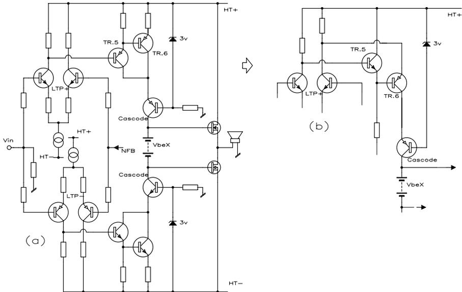
stage were made more sophisticated, with local feedback being added (Figure 4.27 (b)), to enhance linearity.
