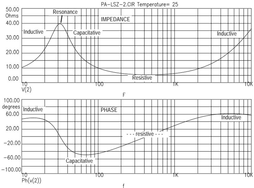
The resonant frequency area(s) of any bass speaker system are commonly highly stressful to amplifiers, and with many BJT amplifiers, when contact is prolonged by a low-enough frequency and perhaps an insistent-enough pounded note, it has frequently been fatal. Other amplifiers have been known to simply burst into uncontrollable oscillation.
