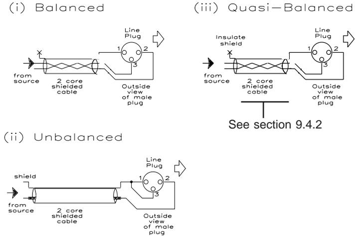
*Female* XLRs (sockets or receptacles) are almost universally used as the chassis mounted input on power amplifiers. There are at least two ways of wiring the incoming male cable plug, assuming one is used per channel.
