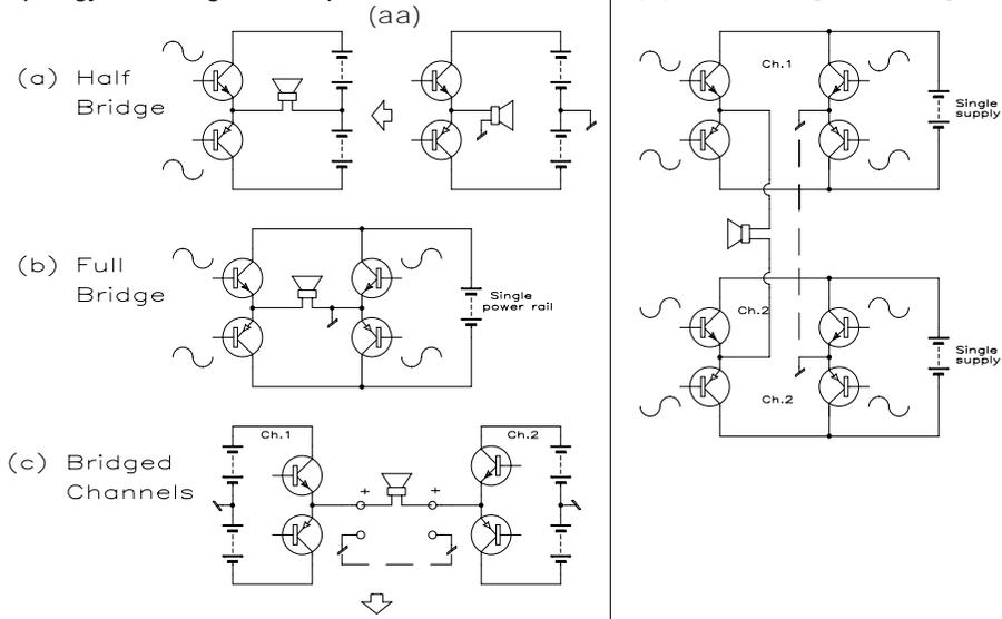
are also driven differentially, as indicated by the sinewave symbols – else there would be no effect. So a third perspective is that we have a balanced (or at least, differential) output also. One feature that is subtly different about Figure 4.34 (b) compared to (c) is that it has just one, floating, power supply. In other words, the bridging of a stereo amplifier with the usual independent, dual supplies is not necessarily the most elegant example of *bridging*.
