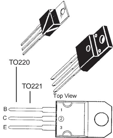
In all cases the central pin is connected to the mounting base or tab.
