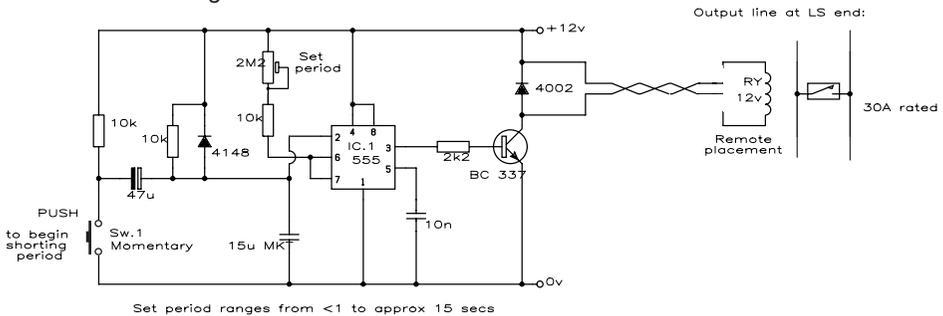
It is little recognised that *even when there is no music signal*, most solid-state power amplifiers can be stressed by (almost) *hard shorting* their output. This because in most designs, DC offset voltage provides a ‘signal’. For example, if there is +50mV DC at the output, and the output’s source impedance is 2mΩ, and the ‘short’ is 35mΩ some way down the wire, then
