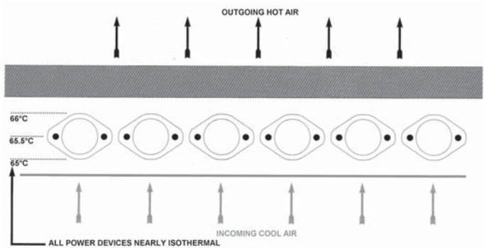
power handling and reliability. Suitably designed short cooling tunnels can also offer isothermal operation.
