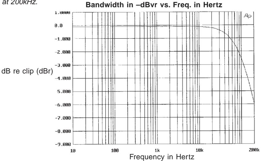
frequencies, this is unavoidable. But there should be no rise ( $+d\text{B}$ ), and no peaks ( $+d\text{B}$ ) nor dips ( $-d\text{B}$ ) in the response, even where rolling-off. As in Figure 7.10.
